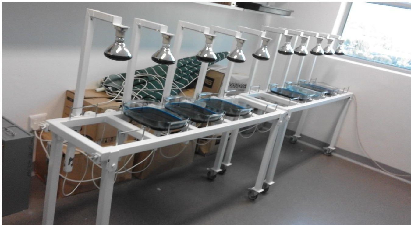
Figure 7: Set up of evaporation pans containing brine-methylene blue solution.
