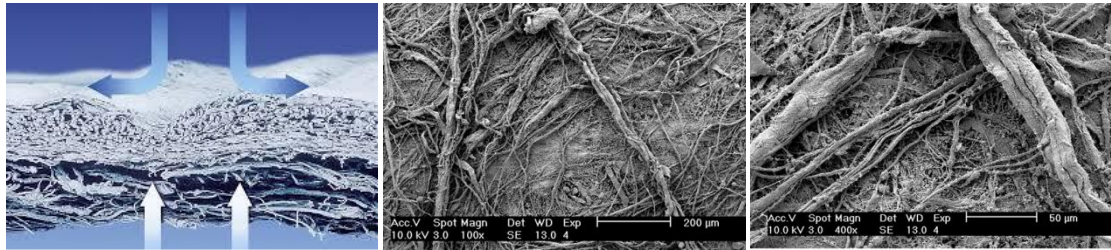
Fig: 2.11. Structure of Bio-Gide®, scanning electron microscopy (SEM) at magnifications of 100x and 400x (adapted from Zhang et al., 2013; Scantlebury & Ambruster, 2012)
