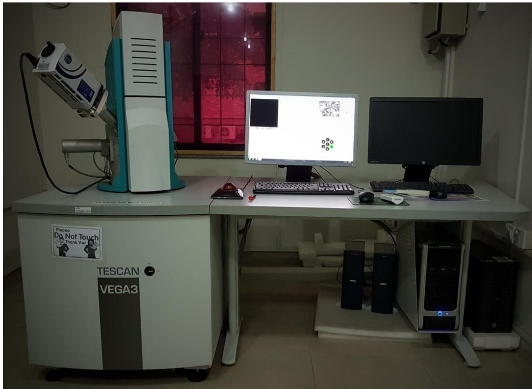
Figure: 4.6. TESCAN Vega3 LMU Scanning electron microscope (SEM) with built-in Energy dispersive X-ray detector (EDX) (X-Act, Oxford Instrument)
