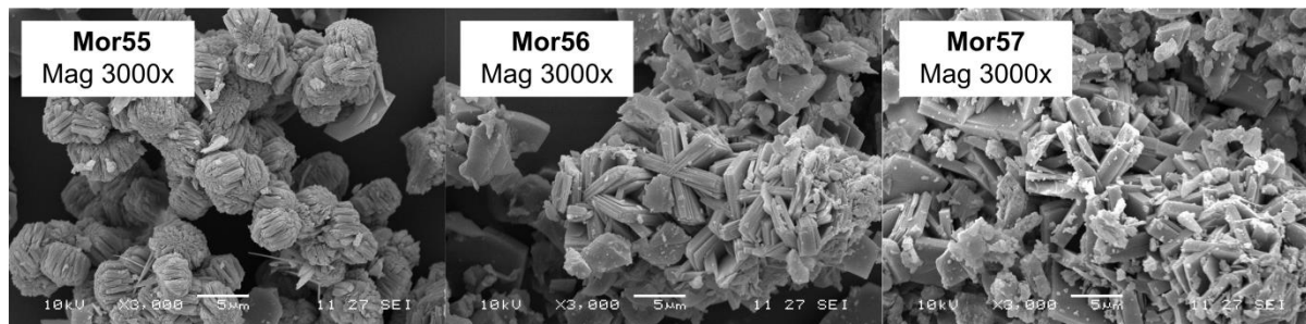
Figure 5.31: SEM micrographs (3000x magnification) of as-synthesised Na-zeolites Mor55-57 synthesised under hydrothermal conditions (170 °C for 72 hours) using varying amounts of ODSA agent (TEAOH), without NaOH or seed crystals added in the synthesis mixture with molar regime in the synthesis mixture with molar regime 1 \text{ SiO}_2 \cdot 0.019 \text{ Al}_2\text{O}_3 \cdot 0.46 \text{ Na}_2\text{O} \cdot n \text{ TEAOH} \cdot 30.1 \text{ H}_2\text{O} ( n = 0.26-1.05 ).
