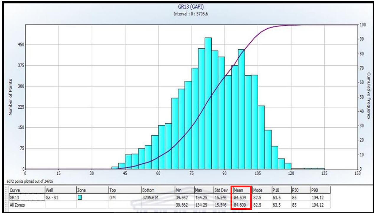
Figure 5.1.2.3: Gamma ray log histogram used to set the baseline for well Ga - S1.
