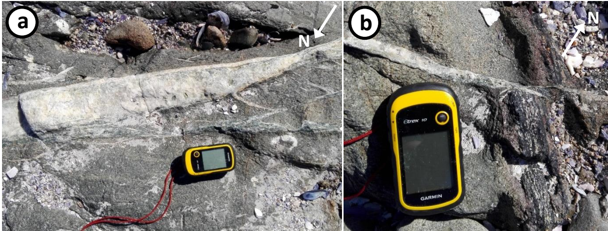
Figure 5.13: ENE-WSW-trending barren quartz veins traversing the monzonite W of the Visitors Center. (a) Quartz vein 2 – 10 cm in thickness and (b) quartz vein 2 – 4 cm in thickness cross-cutting a quartz-pyrite-tourmaline-jasper vein. Scale: GPS with length = 10 cm and width = 5.2 cm.
