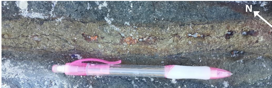
Figure 5.17: WNW-ESE-trending quartz-pyrite vein at Freddie se Klip ranging in thickness between 2.8 and 4 cm. Scale: Pencil with length = 14.5 cm.
