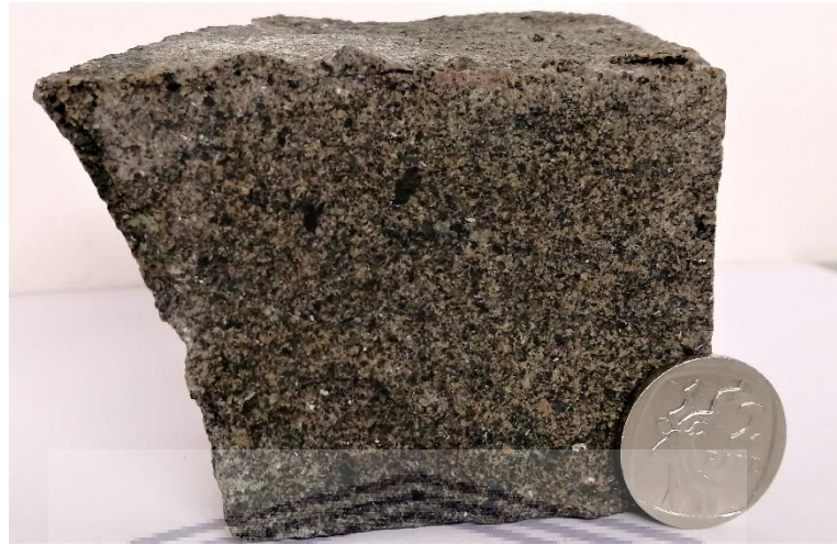
Figure 4.13: Hand specimen of the syenite obtained from Hoëbank (YZN42). Scale: R2 coin with diameter = 2.3 cm.
