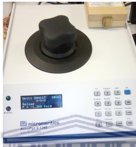
Figure 3.11: Image of the Micromeritics AccuPyc II 1340 helium pycnometer used to measure the skeletal densities of pristine MOFs and MOF composites.
