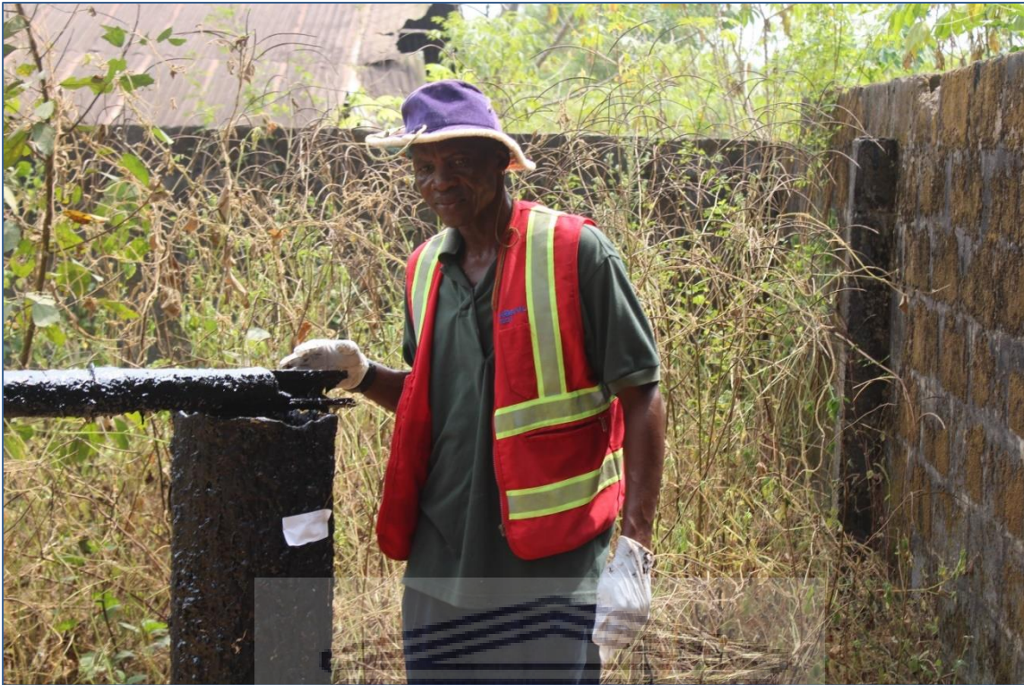
Figure 21: Field photograph showing field assistant at the Agbabu-1 wellhead. The well, now abandoned, encountered heavy oil at a shallow depth. The bamboo wood on top of the wellhead was used to collect heavy oil samples from the well.
