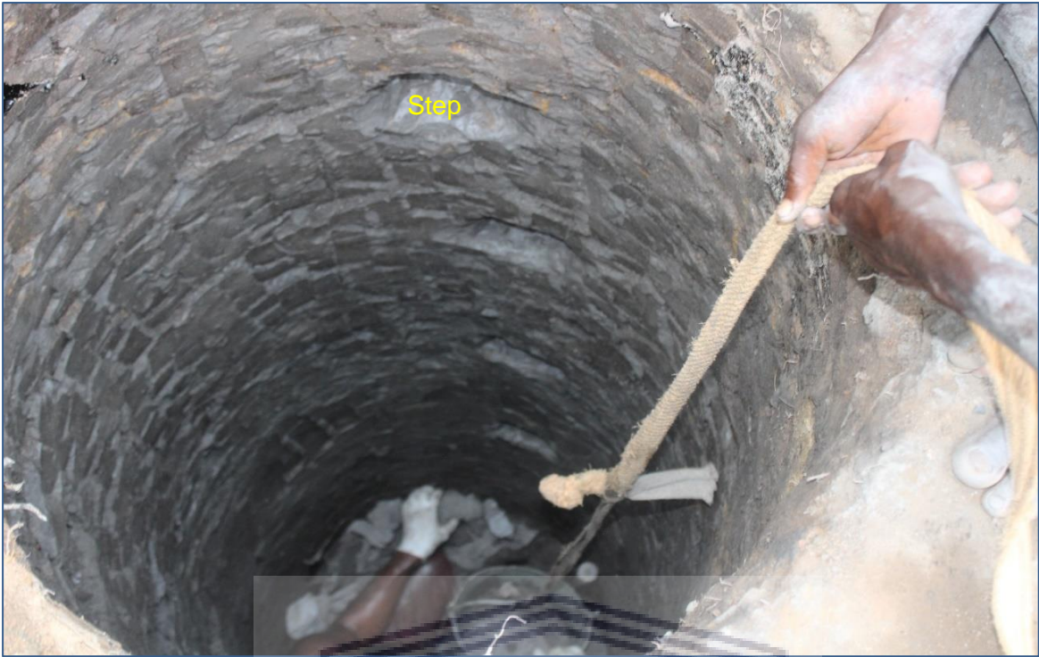
Figure 23: Field photograph showing an intermediate section of J4-BH1. The steps alongside the borehole wall indicated intervals where sidewall samples were acquired.
