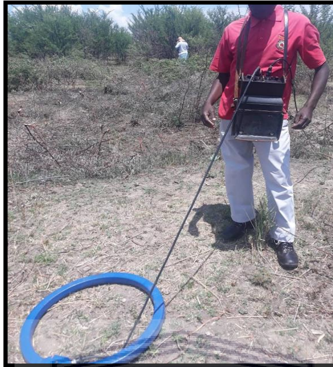
Figure 4.3 Conducting the electromagnetic method with the support of the Department of Water and Sanitation.
