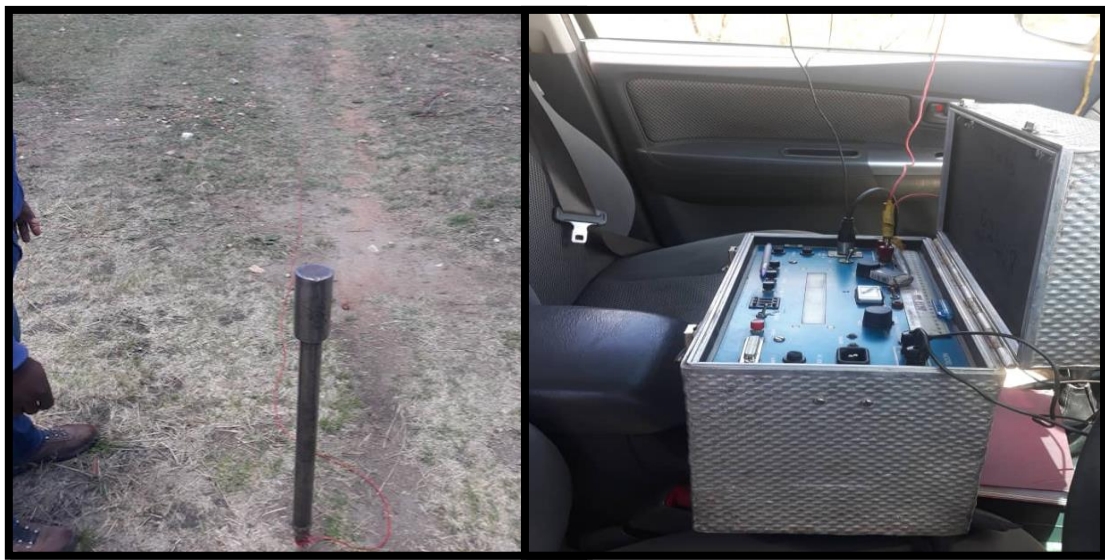
Figure 4.5 Two images display the field set up used for vertical electrical sounding on the experimental sites
