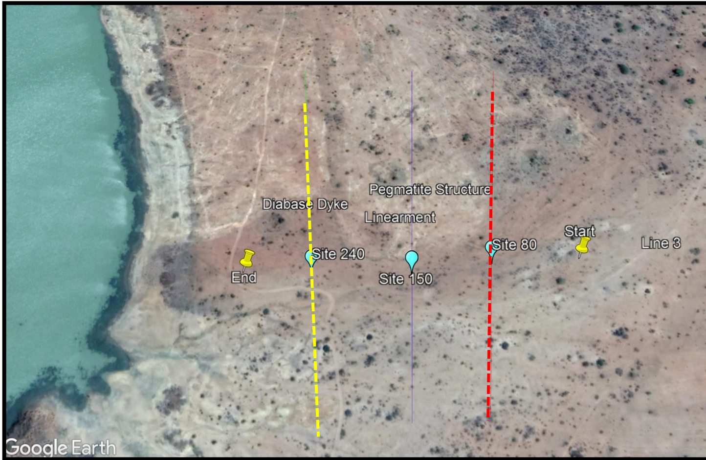
Figure 5.10 Google earth images showing the positions for vertical sounding points for survey region 2 within the study area
