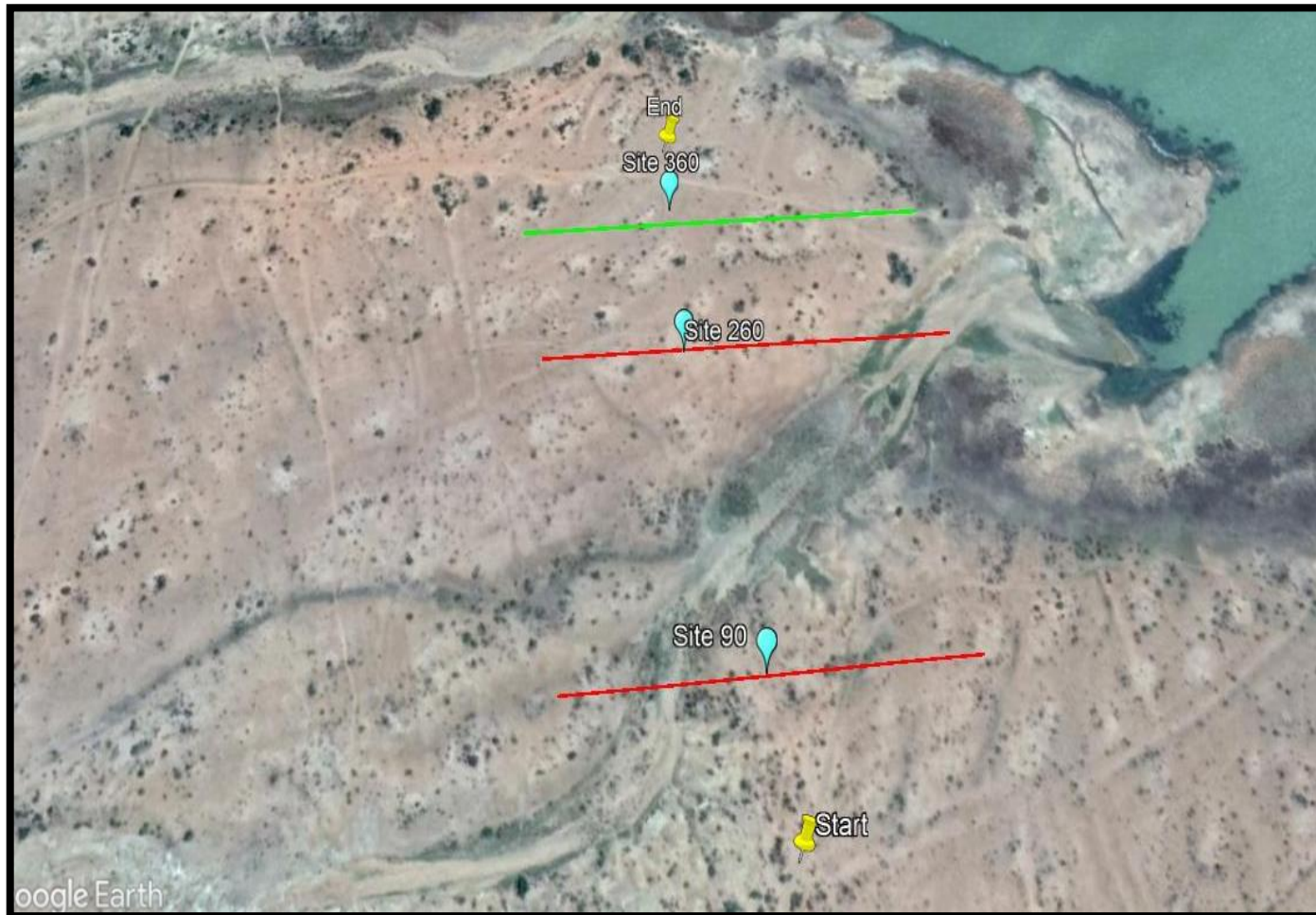
Figure 5.12 Google earth images showing the positions for vertical sounding points for survey region 3 within the study area
