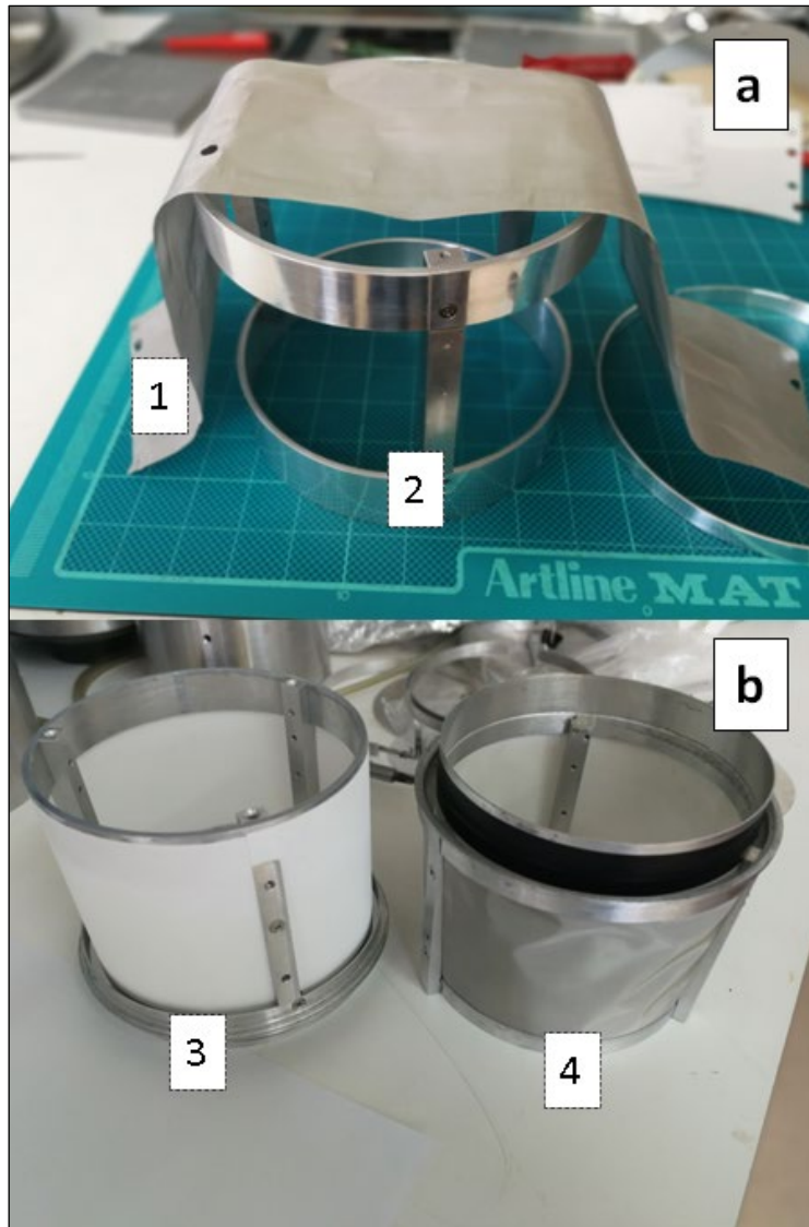
Figure 3-8: (a) Unassembled detector head showing the secondary mesh filter (1) and internal support framework (2). (b) Internal framework with installed white ZnS (Ag) scintillator screen (3) and an assembly with both scintillator screen and surrounding secondary filter (4).
