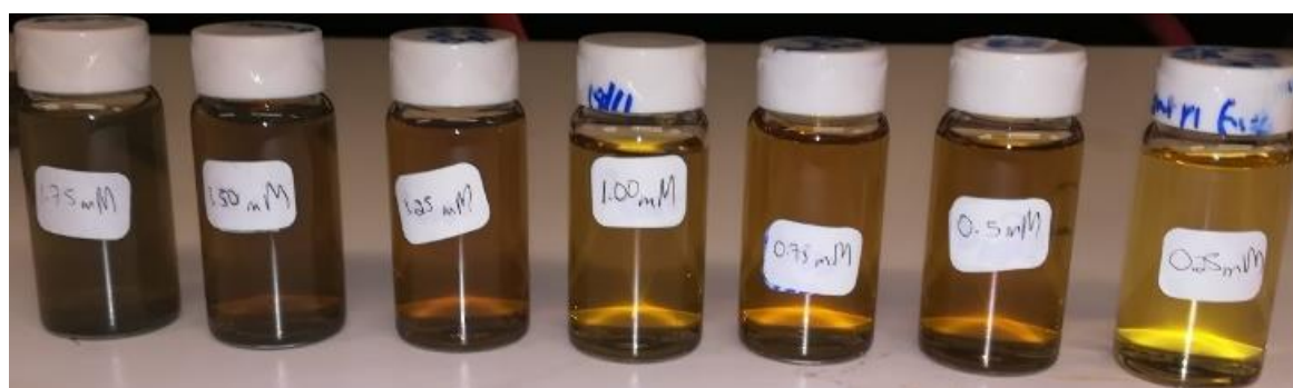
Figure 3. 3: AgNPs prepared by utilizing 0.25, 0.50, 0.75, 1, 1.25, 1.5 and 1.75 mM concentrations of \text{AgNO}_3 , the colour of the prepared AgNPs intensifies with an increase in concentration of the \text{AgNO}_3 .
