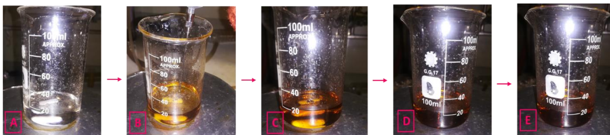
Figure 3. 5: Reaction of \text{AgNO}_3 and \text{NaBH}_4 in the presence of DMSO leading to the formation of DMSO-AgNPs. Different stages of DMSO- AgNPs formation are as follows: (A) reduction, (B) first coalescence, (C) metastable state, (D) second coalescence and (E) final AgNPs.
