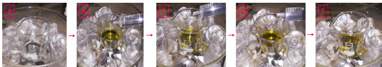
Figure 3. 2: Reaction of \text{AgNO}_3 and \text{NaBH}_4 leading to the formation of bare-AgNPs. Different stages of bare-AgNPs formation are as follows: (A) reduction, (B) first coalescence, (C) metastable state, (D) second coalescence and (E) final AgNPs.
