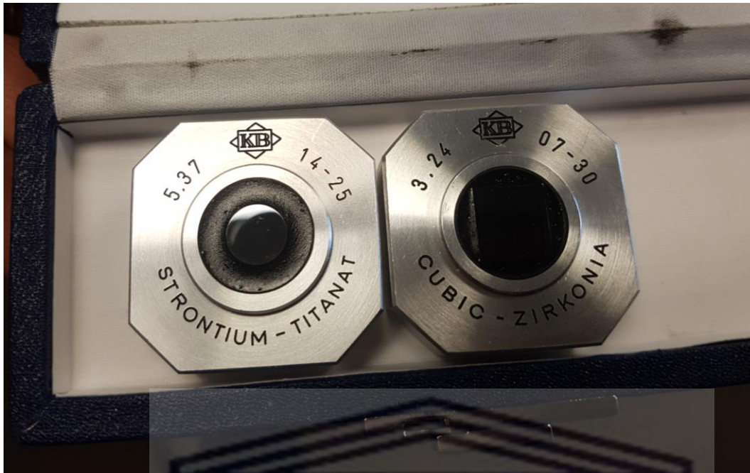
Figure 3.4. Strontium- titanate and cubic- zirconia standards were used for calibration of shale samples.
