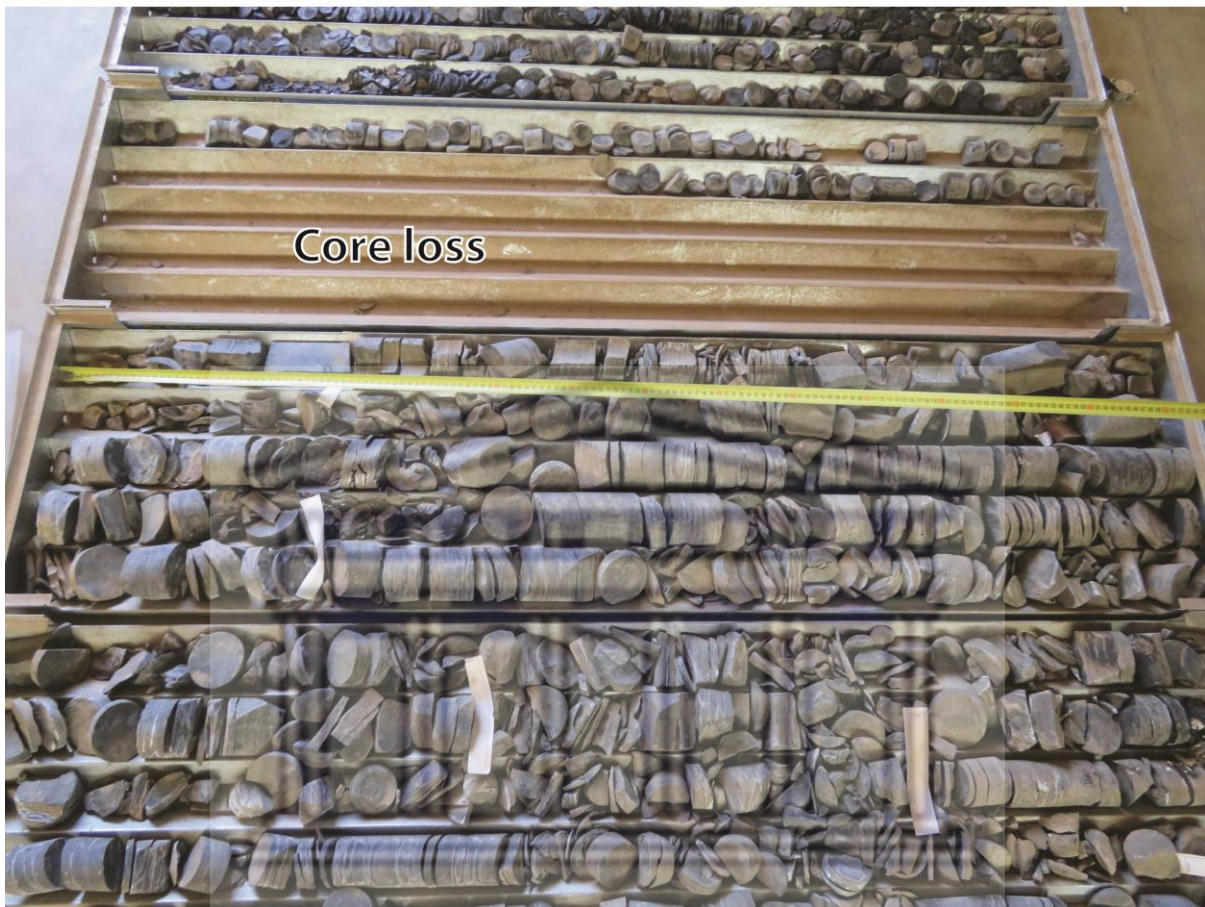
Figure 4.54. Core loss present between depths 2863.55 m and 2879 m underlain by massive shale (Prince Albert Formation) with a core diameter of 6.7cm.
