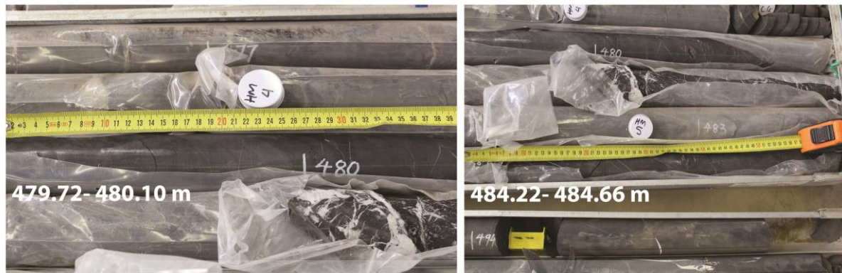
Figure 4.24. Massive shale of the Prince Albert Formation showing positions of samples HM60 and HM61 that were collected respectively from depths 479.72 – 480.10 m and 484.22 – 484.66 m.
