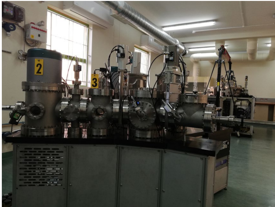
Fig 3.5: Image of the Plasma vapour deposition system used for N 2 treatment
