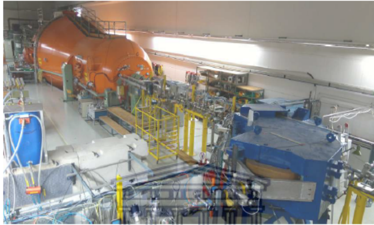
Figure 3.1: A photograph of the tandem hall at MLL, showing the tandem Van de Graaff accelerator (orange) and the 90° analyzing magnet (blue).
