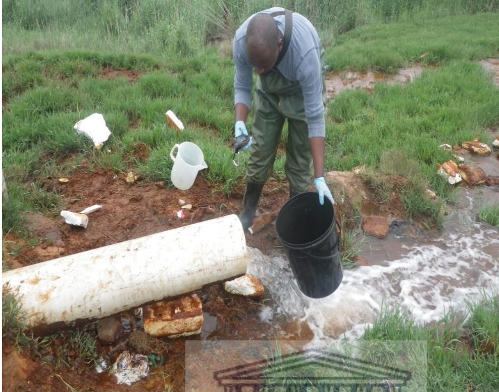
Figure 28: Mine discharge estimation using the bucket and stopwatch method.
