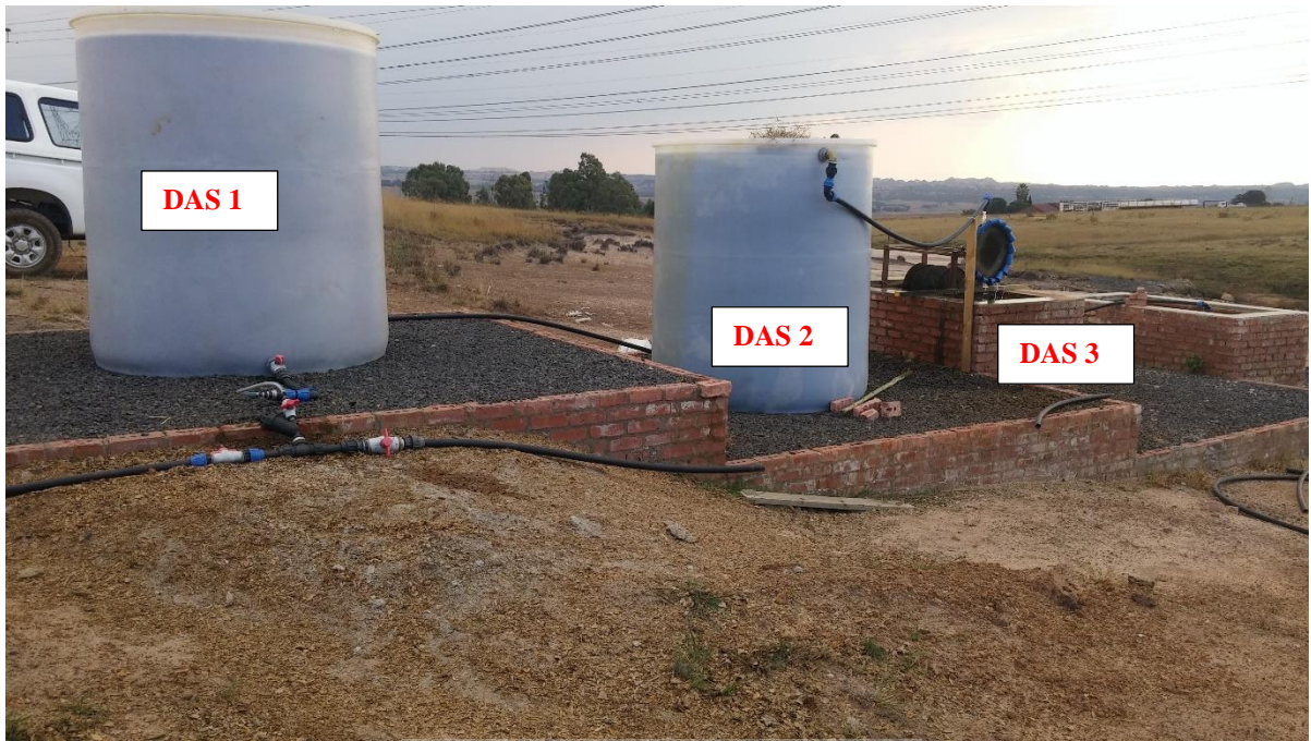
Figure 24: Field-scale set-up of the DAS system implemented at the Douglas site, Mpumalanga.
