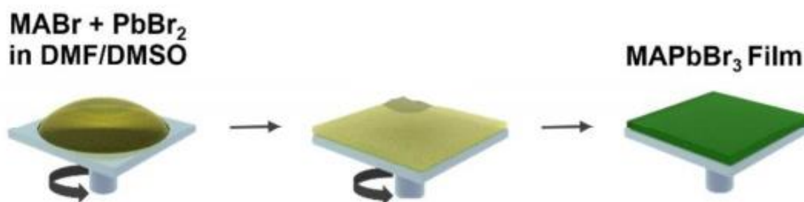
Figure 3.2: Schematic illustration of the spin-coating process for MAPbBr 3 formation
