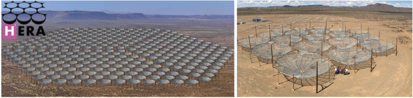
Figure 2.6: Rendering of the 320-element core (left) of the full HERA-350 array and the picture on the right we have on the foreground of 19 HERA 14 m, zenith-pointing dishes (with PAPER elements in the background) currently deployed in South Africa (right) (Deboer et al., 2017)
