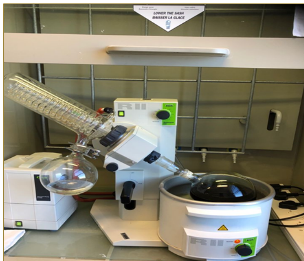
Figure 3.2: Photograph of the Rotovac-Flash evaporator used to evaporate the solvent to yield the crude extracts
