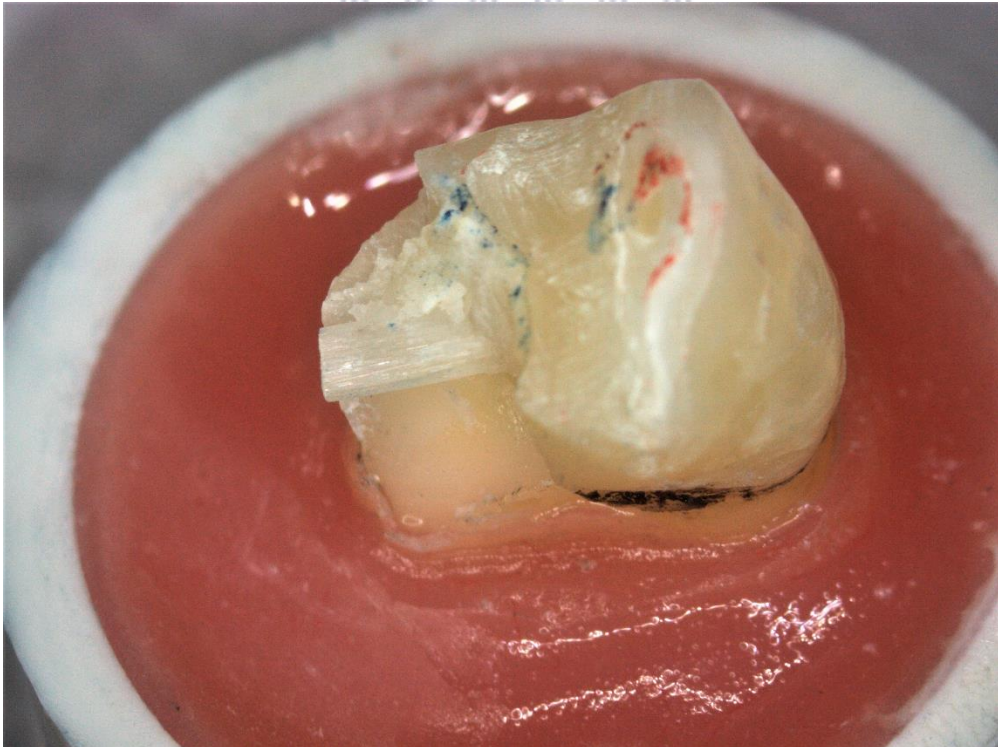
Figure 4.13: Example of mixed failure.
