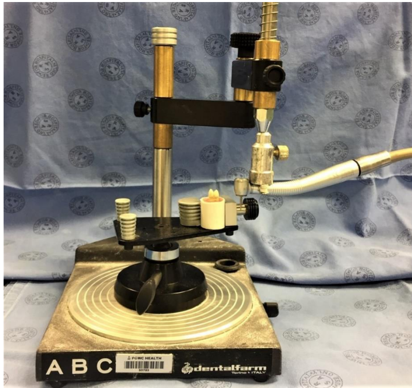
Figure 3.3: Dental surveyor adapted to hold high-speed handpiece parallel to the long axis of the tooth
