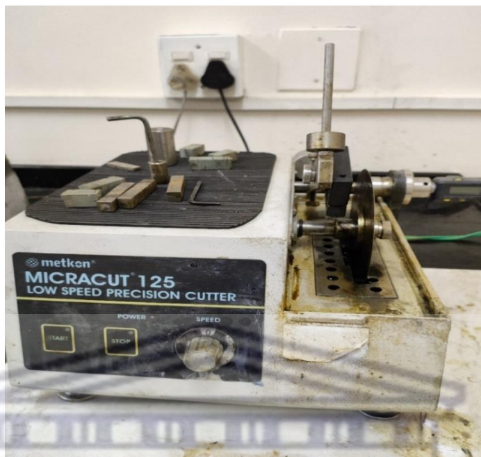
Figure 3.2: Micracut 125 low speed precision cutter with a diamond coated blade of thickness 0.381 mm at the University of the Western Cape.
