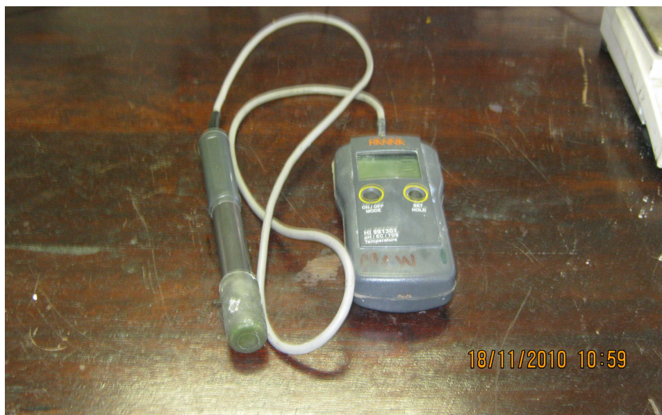
Figure Ai. Hanna HI 991301 pH meter with portable pH/EC/TDS/Temperature probe.
