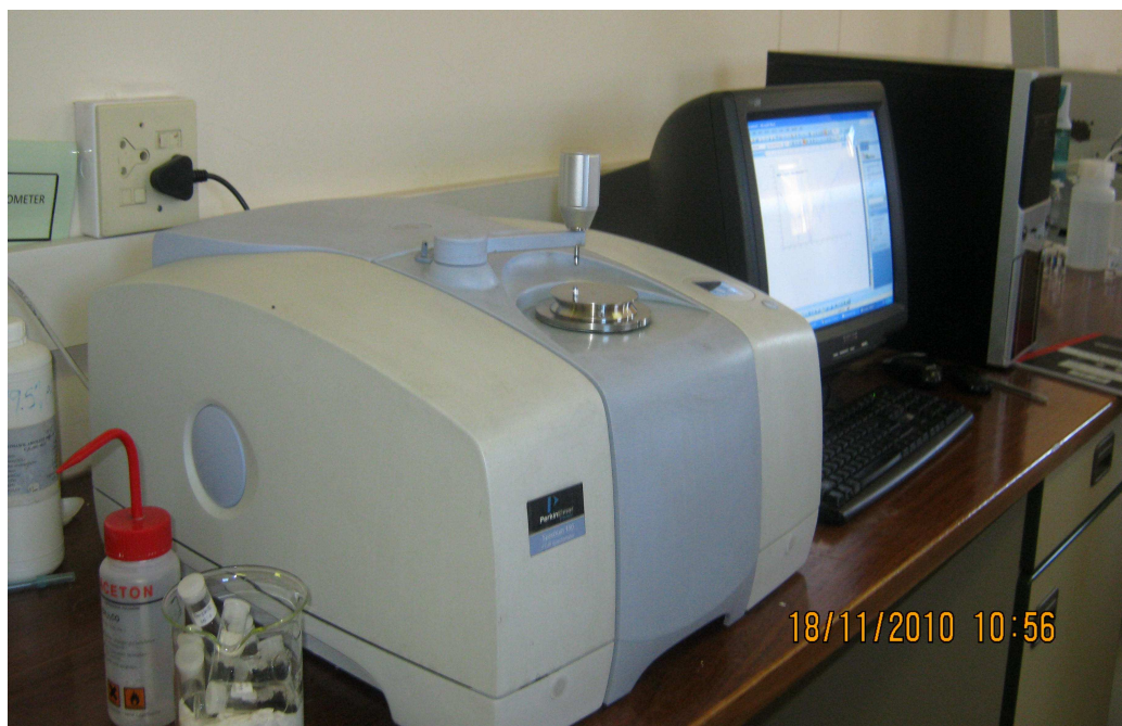
Figure Aiv. Perkin Elmer Spectrum 100 series (FT-IR spectrometer), Universal ATR accessory spectrometer.
