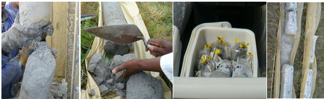
Figure 4.5. Sampling of drilled core ash samples in Zip lock sample bags and storage in a lid plastic container.
