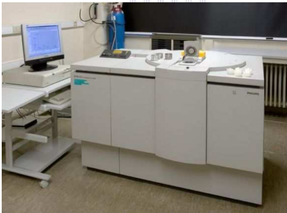
Figure Aii. Phillips PANalytical pw1480 X-ray spectrometry using Rhodium tube as X-ray source.
