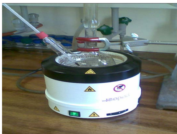
Figure 3.2: Rotating heating mantle and round bottom flask with a thermometer
