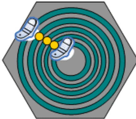
Figure 5.3 Detecting a moving mobile telephone's location by using CGI-TA
