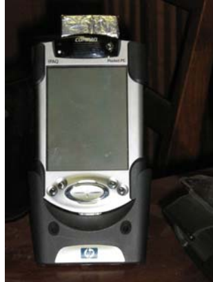
Figure 14: iPAQ h3870 with network card wrapped into an aluminum foil paper
