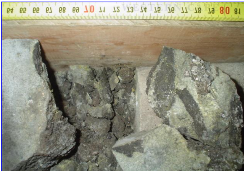
Figure 5.22: Core Photo's of E-M 1 cores 1 and 2, Courtesy of Petroleum Agency of South Africa showing woody material encased within the core unit.
