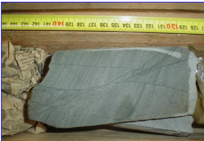
Figure 5.9 Core photo, Core 2 and Courtesy of Petroleum agency, illustrating the orientation or the lack of consistent orientation of the granulation seams.
