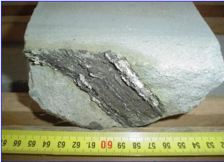
Figure 5.23: Core Photo's of E-M 1 cores 1 and 2, Courtesy of Petroleum Agency of South Africa showing encased woody material in very fine grained sand.
