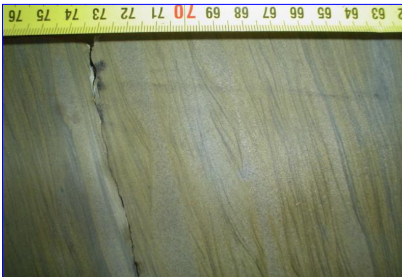
Figure 5.40: Core sample of E-M Suite, Courtesy of Petroleum Agency of South Africa traces of cross bedding visible within core photo.
