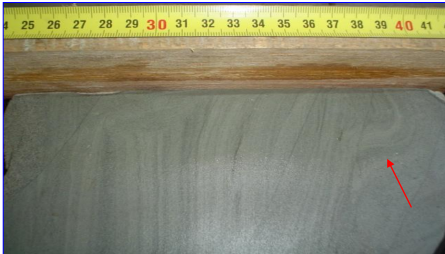
Figure 5.28: Showing a small scale fold indicated by the arrow.
