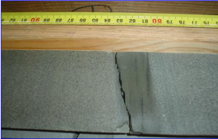
Figure 5.36: Core samples of E-M Suite, Courtesy of Petroleum Agency of South Africa, Occurrence of the interbedded sandstone-siltstone facies which is limited to very thick sandstone intervals.
