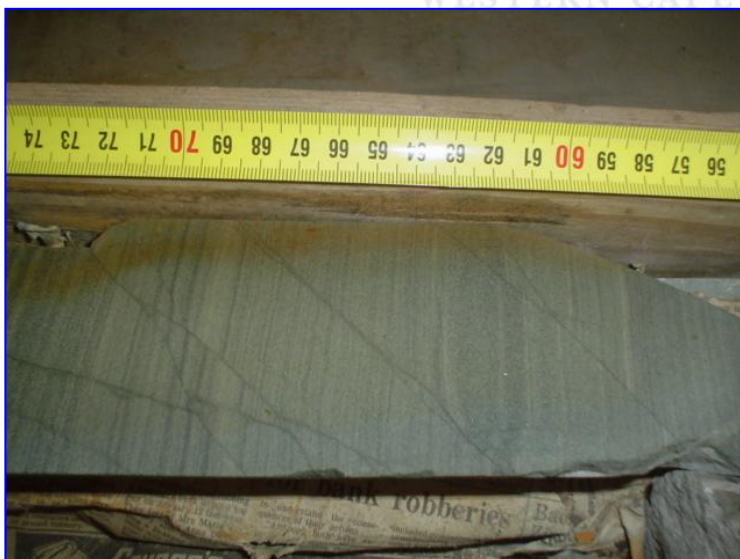
Figure 5.4 Core photos, Courtesy of Petroleum Agency of South Africa E-M2, illustrating the affects of the granulation seams.
