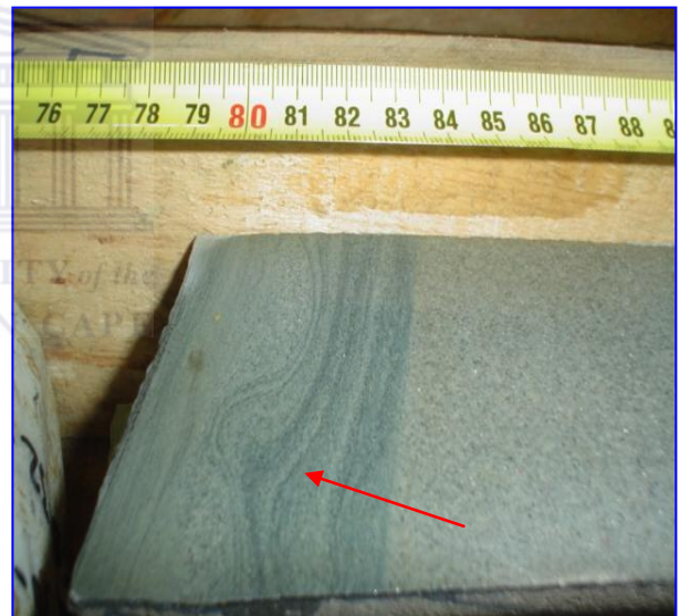
Figure 5.30: Showing dewatering feature indicated with red arrow.
