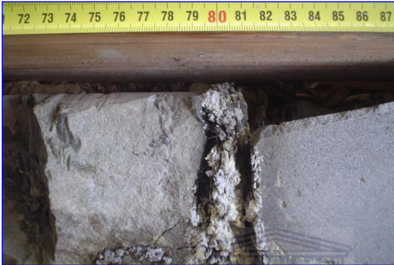
Figure 5.21: Core Photo's of E-M 1 cores 1 and 2, Courtesy of Petroleum Agency of South Africa showing woody material encased in the core.
