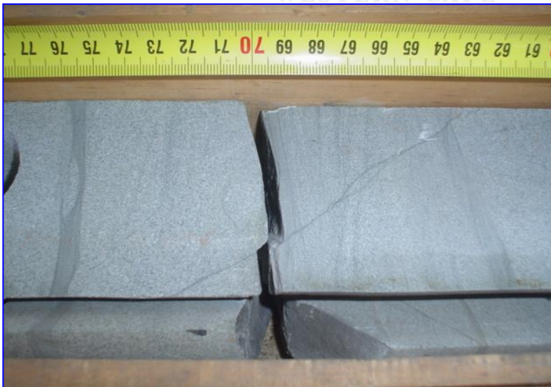
Figure 5.6: E-M 4 Core photo, Courtesy of Petroleum Agency of South Africa illustrating the affects of the granulation seams.
