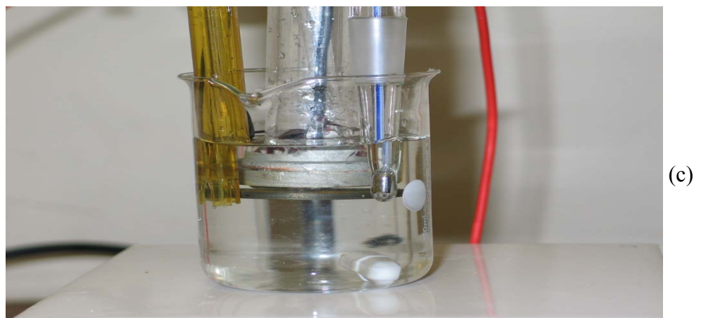
Photographs 3.1. Fe/O 2 battery experimental set up (a), (b) and (c)
