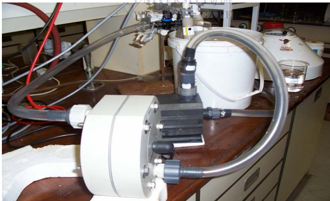
Photograph 4.1 Electrolyser Diacell ® (type 106:01-010)
