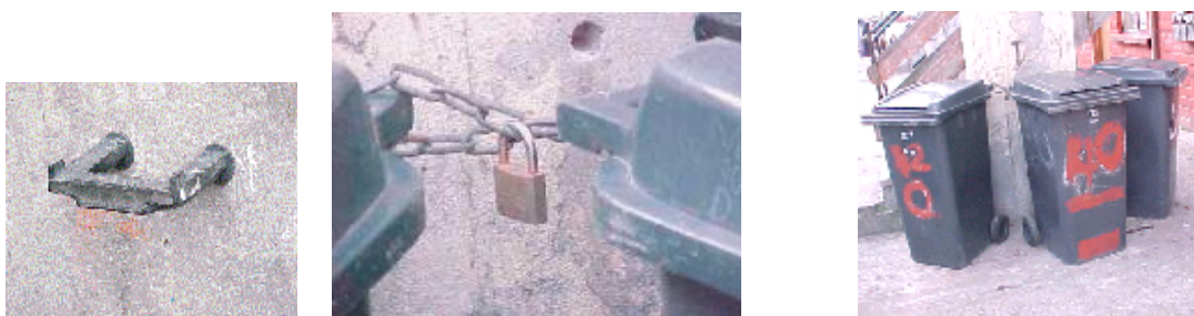
Plate 11: Device used to secure bins on ground floor of flats
