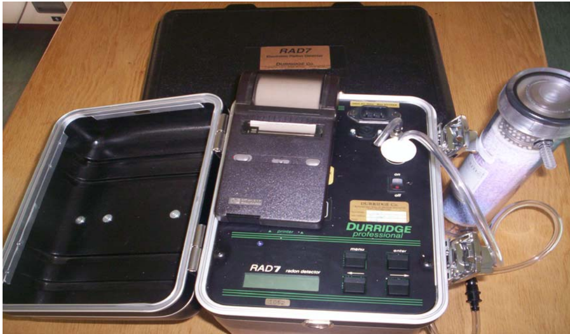
Fig 4.2: Radon continues monitor (RAD7)
