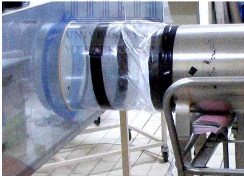
Figure 5: The isolator joined with the food autoclave unit by a transfer tunnel.
