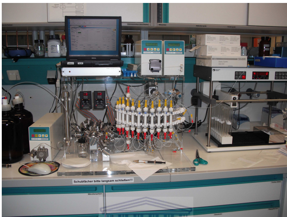
Plate 2. Medium Pressure Liquid Chromatography equipment (MPLC) used at GeoForschungsZentrum (GFZ), Potsdam, Germany
