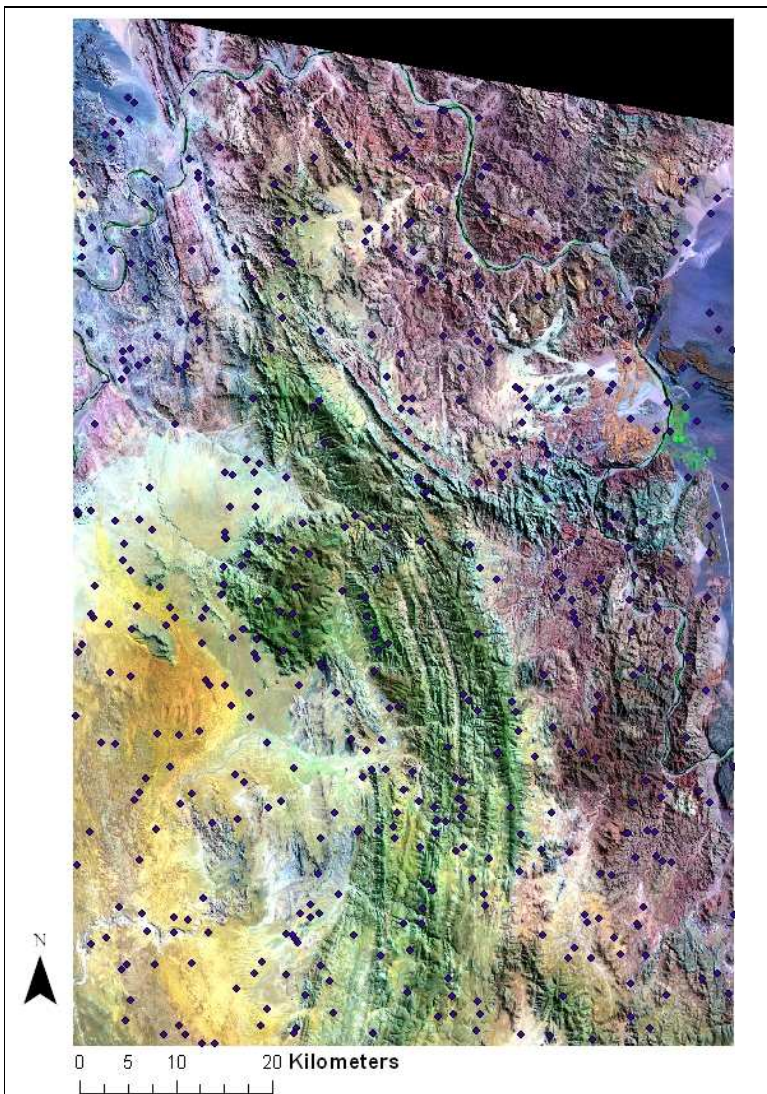
Figure 5: A 30m Landsat image (band combinations: R:3,G:4,B:1) showing the study area, as well as the random validation points used in the accuracy assessment.
