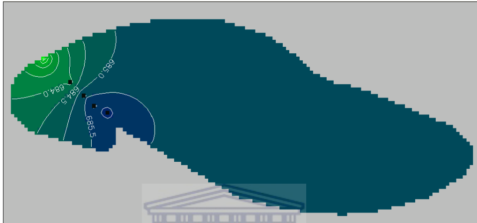
Fig. 6-28 Initial hydraulic heads in the modeling area
