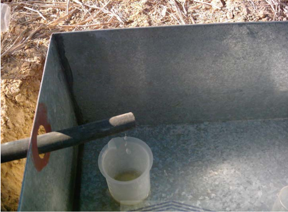
Figure 6.3 illustrating the occurrence of the first run-off
