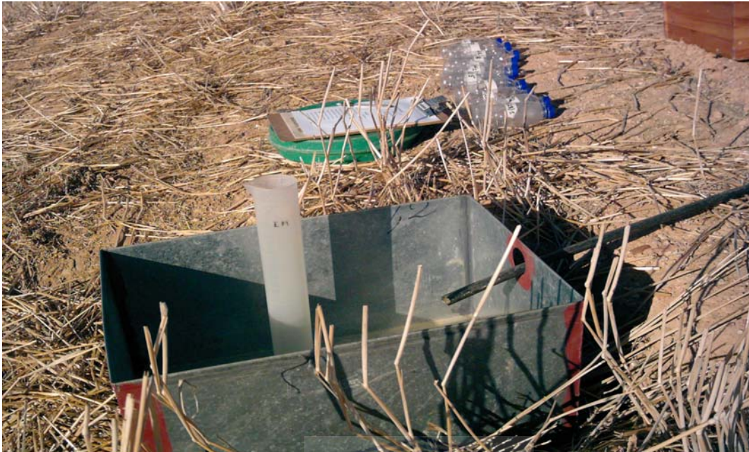
Figure 6.5 illustrating sample bottles, cylinder to measure the run-off, metal container to collect run-off, paper form for recording the data, wooden box to keep the samples
