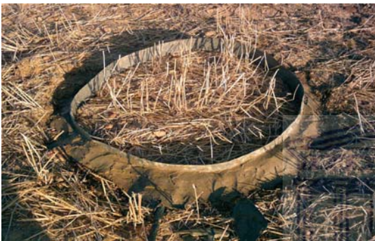
Figure 1.2 Metal ring-enclosed surface with 75% coverage of wheat stubble (photo courtesy of Willem de Clercq)
