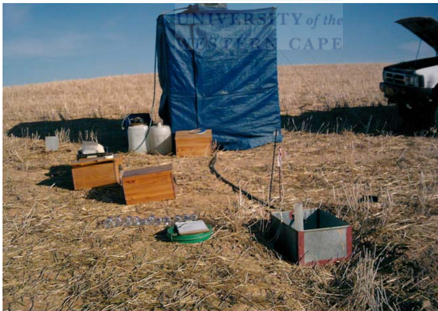
Figure 6.2 illustrating different equipment used during rainfall simulation, canes containing water and wooden boxes for samples
