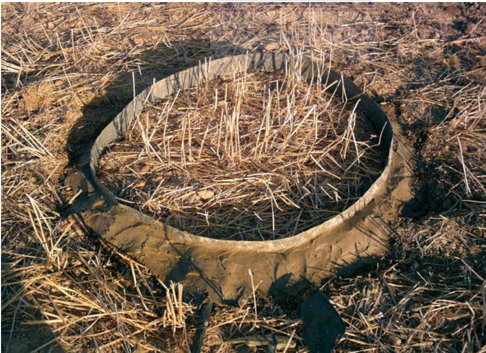
Figure 3.2 Indicates simulation ring over stubble land
