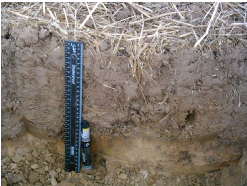
Figure 1.4 Soil horizon indicating the upper 300 mm from where samples were collected
