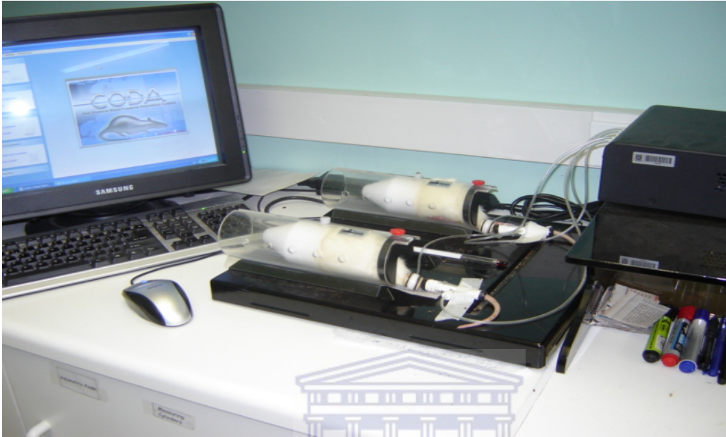
Figure 3.2: Non-Invasive Blood Pressure system showing the rats in rodent holders on a heating stage to increase blood flow to the tail.
