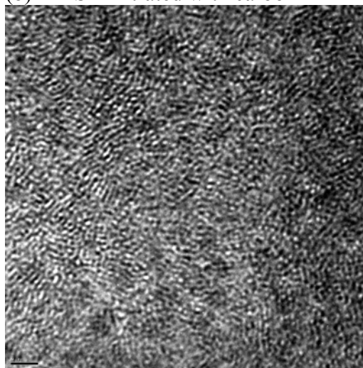
(d) HRTEM of OMC showing wormhole pore structures analogous to HMS
