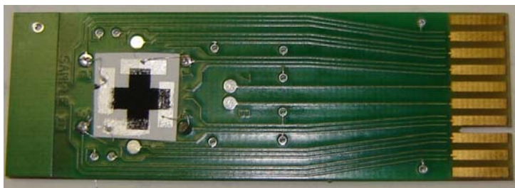
(a) Indium contacts for samples overprinted onto silver printed contacts on Lakeshore Sample Holders 750SC10-50
