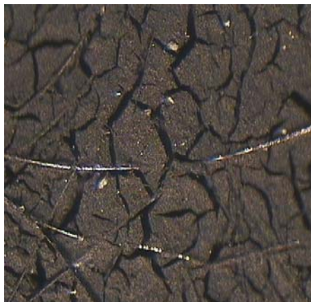
Figure 7.15 Optical microscopy of typical composite electrode JM Pt 40 /C on carbon cloth
