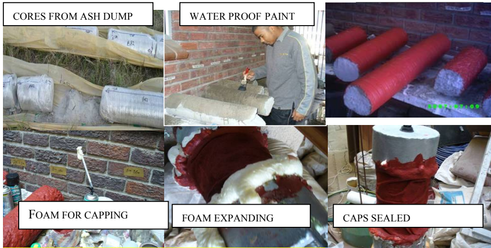
Figure 4.14 Sample preparation of cores for laboratory hydraulic and tracer testing.
