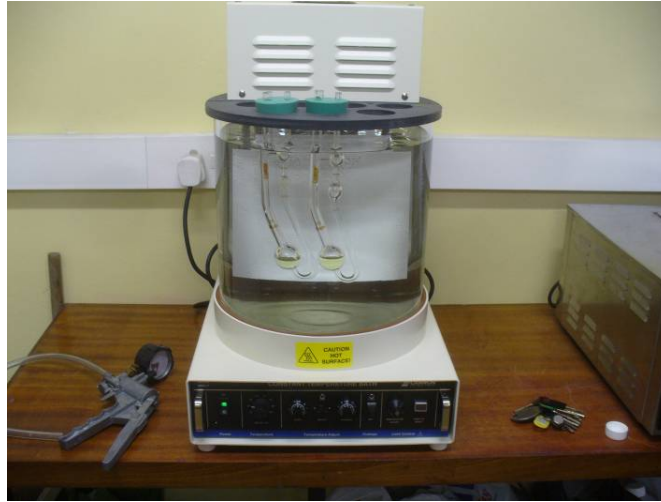
Figure 4.3 Viscosity and Liquid Density measurements performed under constant temperature of 30 degrees.
