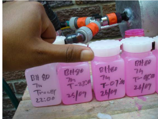
Figure 4.17 Qualitative display of tracer breakthrough, lighter colors are observed for the first sample and darker colors are observed with time.
