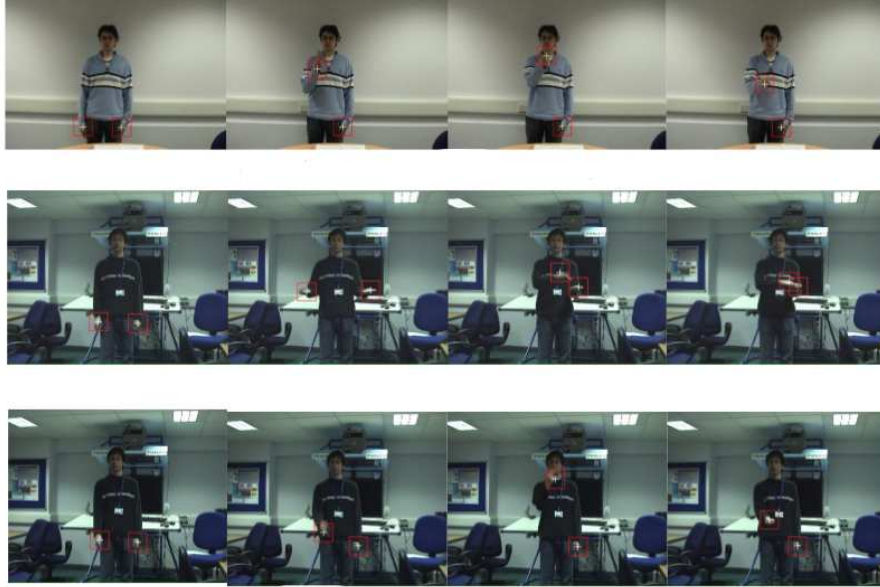
FIGURE 2.23: The tracking of both hands, but not distinguishing between them using the framework of Ongkittikul et al. [120] (p. 205).
