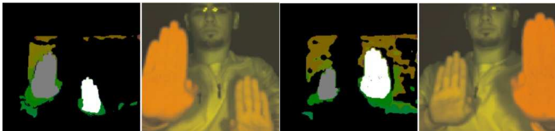
FIGURE 2.14: The depth data are used to track the hands, where the grey and white clusters represent the right and left hand, respectively [27].
