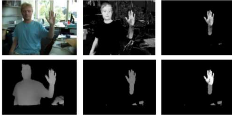
FIGURE 2.1: Using depth data (bottom left and bottom middle) and skin-colour information (top middle and top right) to find a hand (bottom right) [156] (p. 68).
