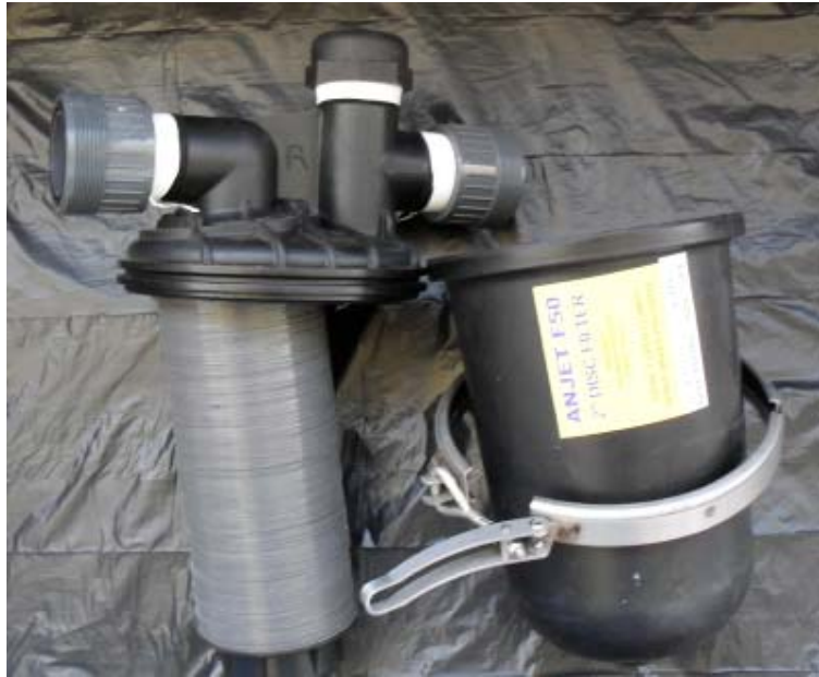
Fig. 7.9 The ANJET F50 disc filter that replaced the sand filter.
