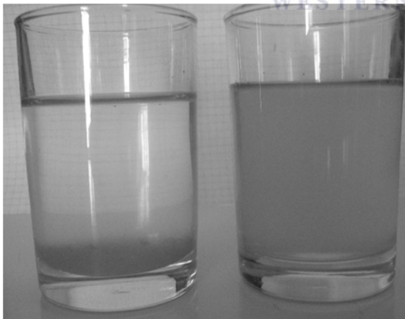
Fig. 5.9 Turbid water from the site. Left: After 5 days standing (~10 FNU). Right: fresh from the tap (~120 FNU).
