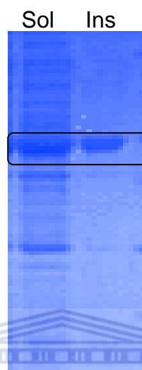
Figure 4.18: Analysis of the soluble and insoluble protein fractions after optimisation of expression (25 °C, 1 mM IPTG, 5 mM divalent metal ions. Sol: soluble fraction, Ins: insoluble fraction. Band predicted as hydantoinase circled in black box.
