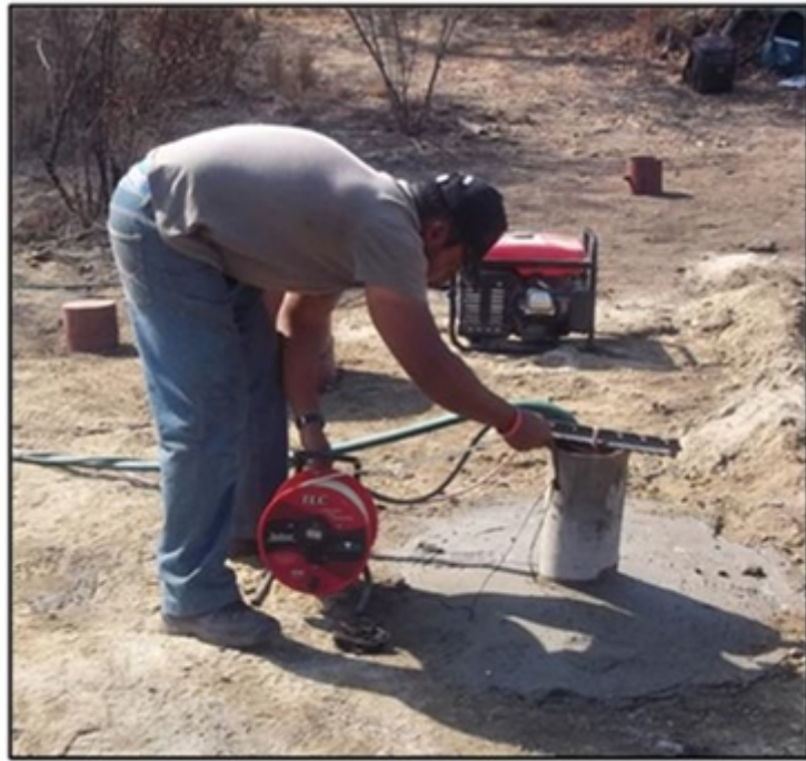
Figure 4.6 Use of a Solinst TM water level meter to measure groundwater level at an error of \pm 0.02 m.
