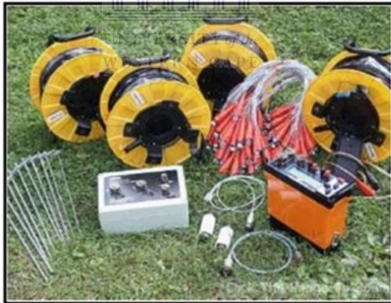
Figure 4.1 An Abem Signal Averaging System (SAS) 1000/4000 Terrameter and switching unit powered by a 12 volt battery with 64 steel probes and clips to connect to four 100m cables with 21 take outs on each to form electrodes.
