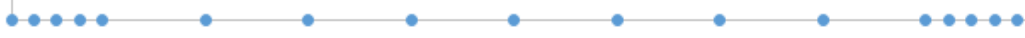
Figure 1.6: Shishkin mesh for a case with boundary layers near x = 0 and x = 1 .
