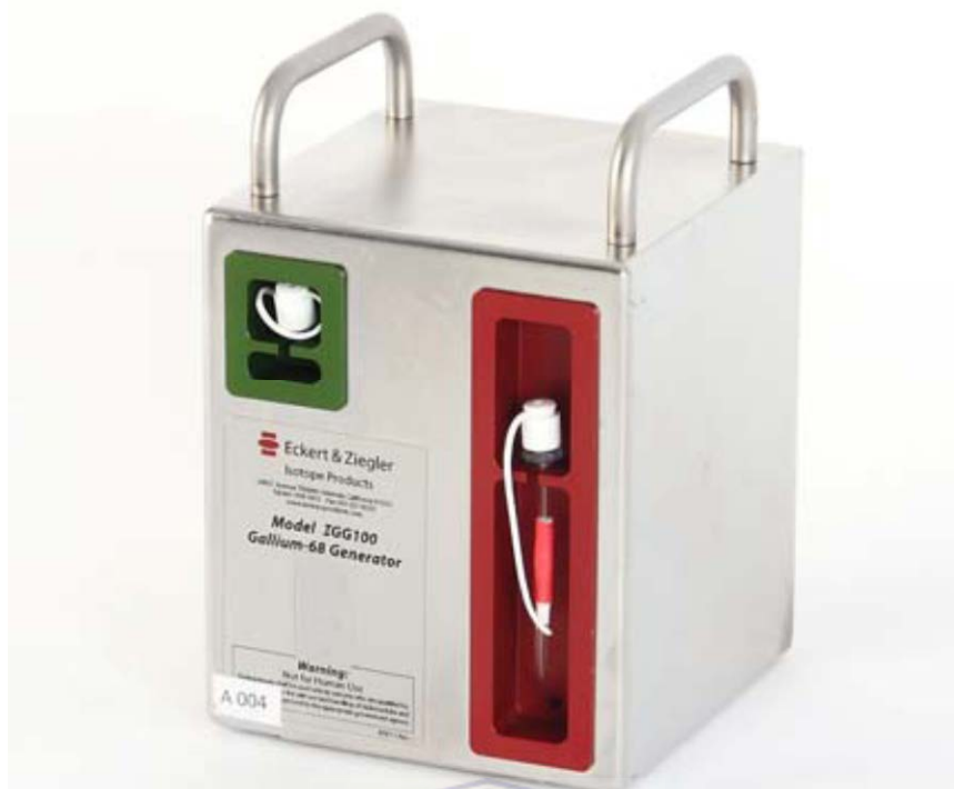
Figure 2.7: An Eckert and Ziegler Isotope Production ^{68}\text{Ge}/^{68}\text{Ga} generator, Berlin
