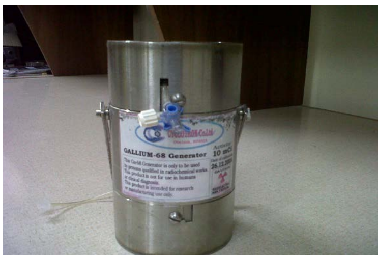
Figure 2.6: A 10 mCi (370 MBq) commercial \text{TiO}_2 generator from Obninsk, Russia by Cyclotron Company Limited
