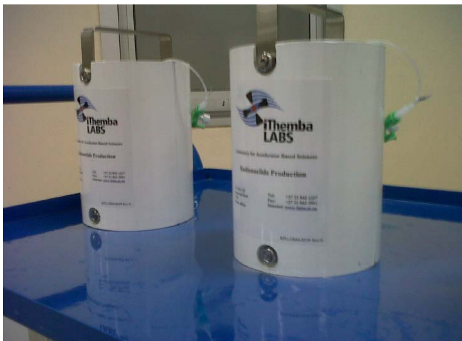
Figure 2.9: iThemba LABS SnO 2 based 68 Ge/ 68 Ga generator (Somerset West, South Africa)
