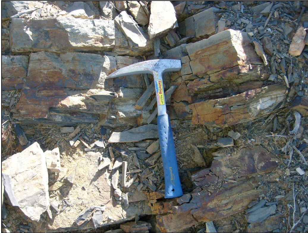
Figure 4.8. Brown weathered resistant cherty and/or micaceous shale of the upper Whitehill Formation.
