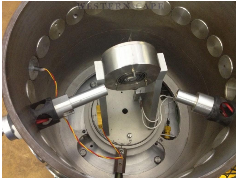
Figure 3.7. A RT-ERDA set up at iThemba LABS for isochronal annealing of a -SiC:H films.
