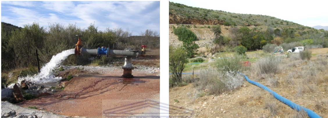
Fig. 6.13: Artesian borehole C1b3 in Oudtshoorn and the free-flowing test conducted from late September till November, 2009 (Hartnady et al., 2013)
