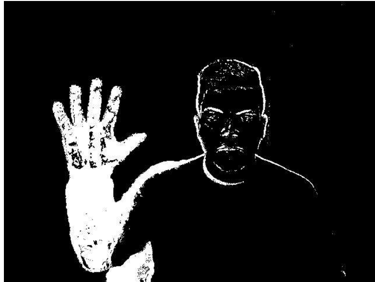
FIGURE 4.4: The result of applying Gaussian Mixture Models to highlight moving pixels—the motion image.
