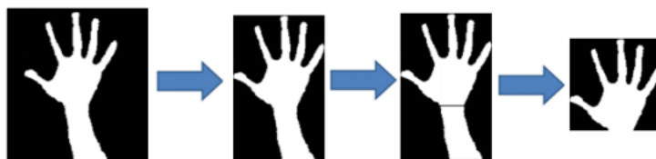
FIGURE 2.6: Segmentation of the hand from the arm [46].
