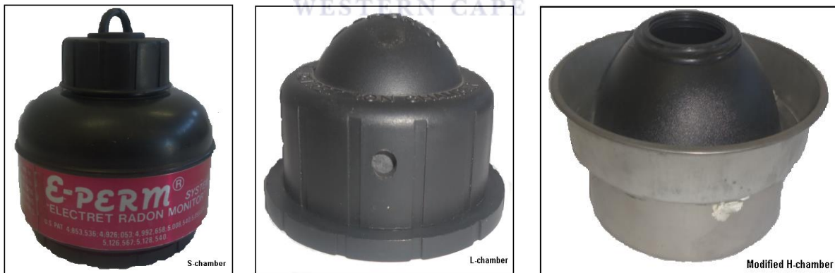
Figure 5.12: A picture of a closed S-chamber on the left, L-chamber in the middle and the H-chamber on the right. The latter is shown in the adapted form used for flux measurements.
