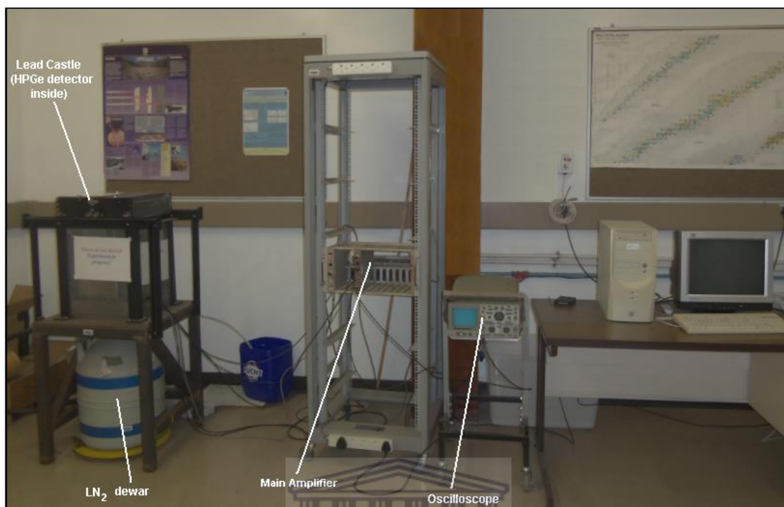
Figure 4.18: A picture showing the set-up of the HPGe detector system comprising of the lead castle, the liquid nitrogen dewar and the other components of the system.
