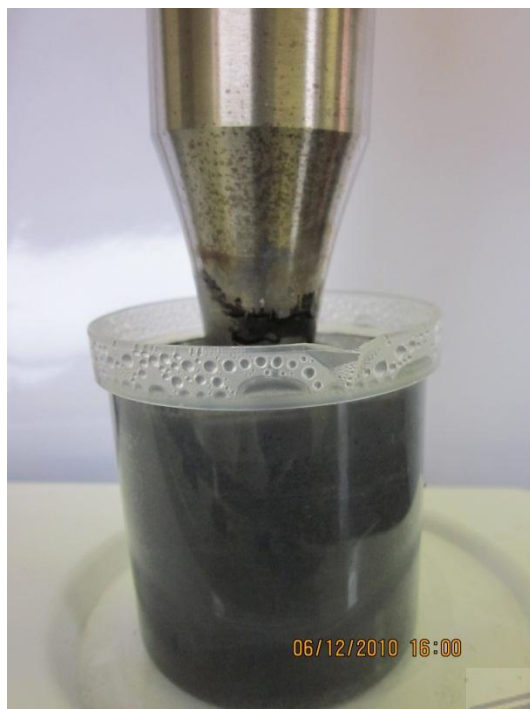
Figure 3-13: Standard ultrasonic processing tip (3/4'') inserted in the synthesis mixture.
