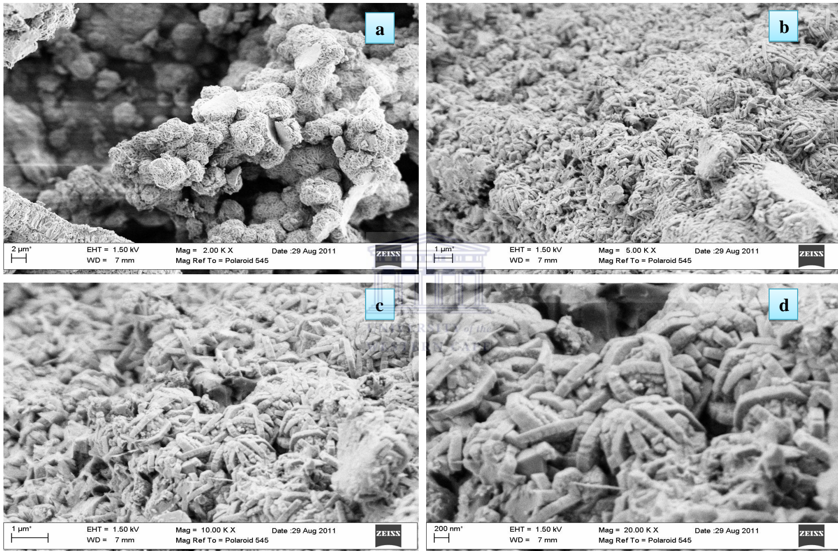
Figure 5-14: SEM micrographs of hierarchical zeolite X synthesized from clear fused fly ash extract at 94 °C for 24 hours (Con X94) - shown at different magnifications a) x 2,000 b) x 5,000 c) x 10,000 and d) x 20,000.
