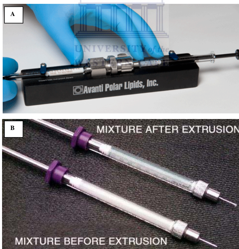
Figure 1.19 Avanti® Mini-Extruder. Extruder compartments include two gas-tight glass syringes, membrane compartment and a heating block (A). The more times the liposome suspension passes through the membrane, the more homogenous the lipid solution becomes, as noted by the whitish colour of liposome suspension before extrusion and the more transparent liposome suspension after extrusion (B) ( http://www.avantilipids.com/index.php?option=com_content&view=article&id=533&Itemid=297 ).
