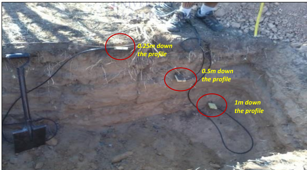
Fig. 3.5 Soil profile pit showing soil sensors monitoring the volumetric soil water content at different depths down the soil profile.
